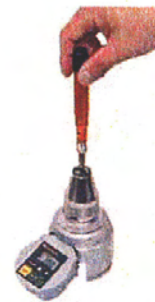
Torque checking figure for BMRD torque screwdriver for small screws with BTGE-G
