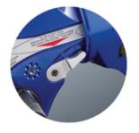
The MXT was the first tool in the industry to feature a release lever that allows you to release the tool if it locks on the application. (Also found on Avanti series)
