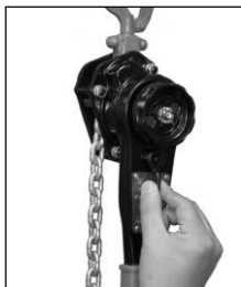
1) Set the selector lever to "N" position.
