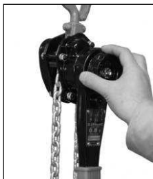
2) Turn the feed handle half-turn counterclockwise. Then, free spooling will be available automatically.
