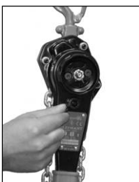
4) Set the selector lever to "UP" position.
