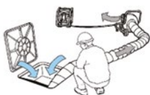
Aspiration in manholes and closed ambients
