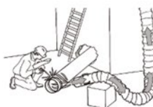
Suction of welding fumes in indoor works
