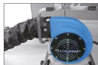
Detail of the quick installation system of the hoses on the tool mouth
