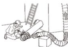
Suction of welding fumes in indoor works
