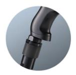
The Digital jGun is the first of its kind with an onboard air regulator for simple torque adjustment with a twist of the connector at the bottom of the handle. Especially convenient when switching from tightening to loosening, giving you the ability to quickly adjust to full power for fast and easy break-out.
