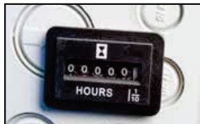
Hour meter to help on maintenance controls and rental fleets.
