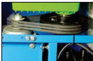
New easy and quick belts tightening system.
