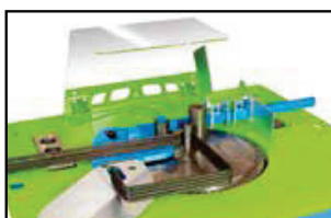
Stirrup device for max. rebar Ø 14mm / 5/8" - #5 (optional).
