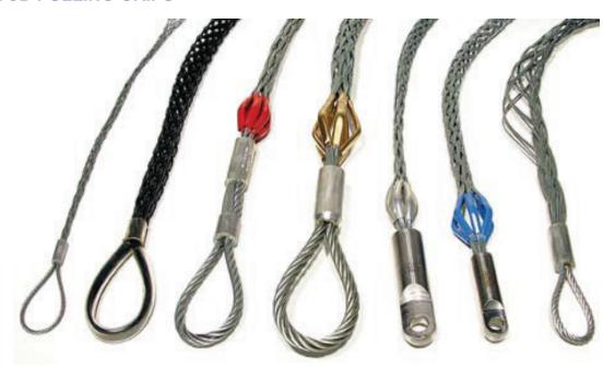
DCD cable grips are hand-woven by experienced trades people guaranteeing a consistent level of high quality. DCD grips are reverse woven, creating a loop at the end of the grip instead of being soldered or crimped together (see photo inset left of typical grip end).
