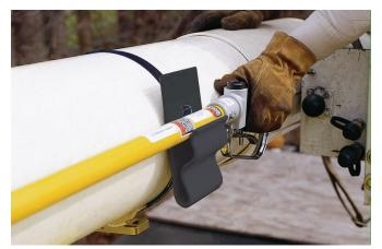
Handle Unit Included With All Boom Mount Tool Holders Ratchet strap fastens handle holder securely into a fixed position on the boom. Its rubberized coating prevents tool handle from sliding out of the upper holder box. Fits round and square booms.
