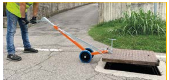
Use 3: mechanical opening with locking clamps.
