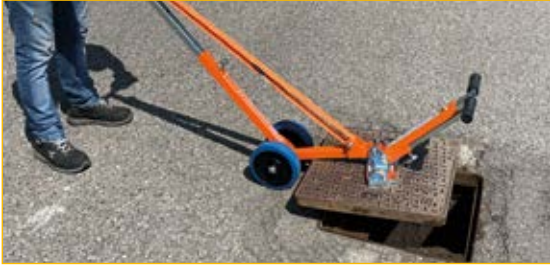
Use 1: opening with magnetic CL9 - CL10 - CL11.
