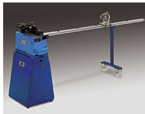
UNI 60 electric, complete with moving plane of bend and universal base.
