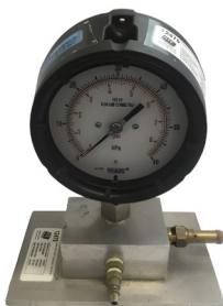
Test Gauge for Pipeline Pressure Testing
