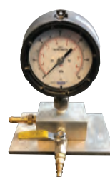
Test Gauge for Pipeline Pressure Testing
